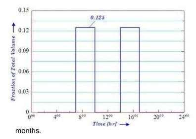
If the household uses the same volume of water but a different pattern as indicated in the adjacent figure between 7 a.m. and 9 a.m. and from 1 p.m. to 5 p.m., the annual energy saved and the NPV are less and the payback period is more: 6 years and 3
