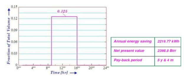
If the utilisation of the water is such that it is distributed over the day from 9 a.m. to 4:00 p.m., in other words 12.5% of the volume of water will be utilised by the household. The annual energy saving as a result of this pattern of consumption by the household is 2219/77 kwh. The NPV for this pattern is 2398.8 Birr and the household will get their investment payback in 5 years and 4 months time.
