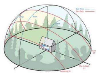
mechanism from East to west, this should be carefully considered when placing collectors to trap as much energy as possible. The technique is that SWHs in the northern hemisphere should be facing south and SWHs in the southern hemisphere should be facing north. In the case of Ethiopia, as we are located 9 Degrees north of the equator (Addis Ababa), SWH collectors should be facing south.
