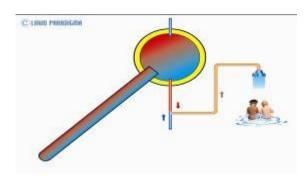
As the key components of the solar collector, the evacuated tube is a product optimised in geometry and performance. The tubes are composed of two concentric glass tubes which in each case are half spherically closed on one side and fused together on the other side. The gap between the tubes is evacuated and afterwards hermetically plugged (vacuum installations). In order to make solar power usable, the internal glass tube is provided on its external surface with an environmentally friendly,
